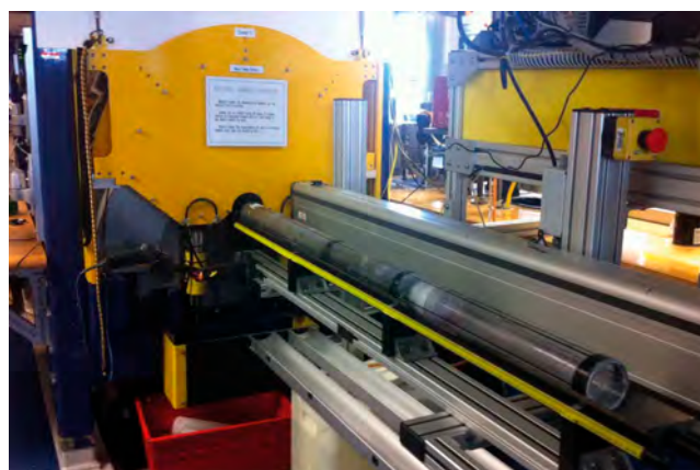
Figure F17. Natural Gamma Radiation Logger (NGRL).
