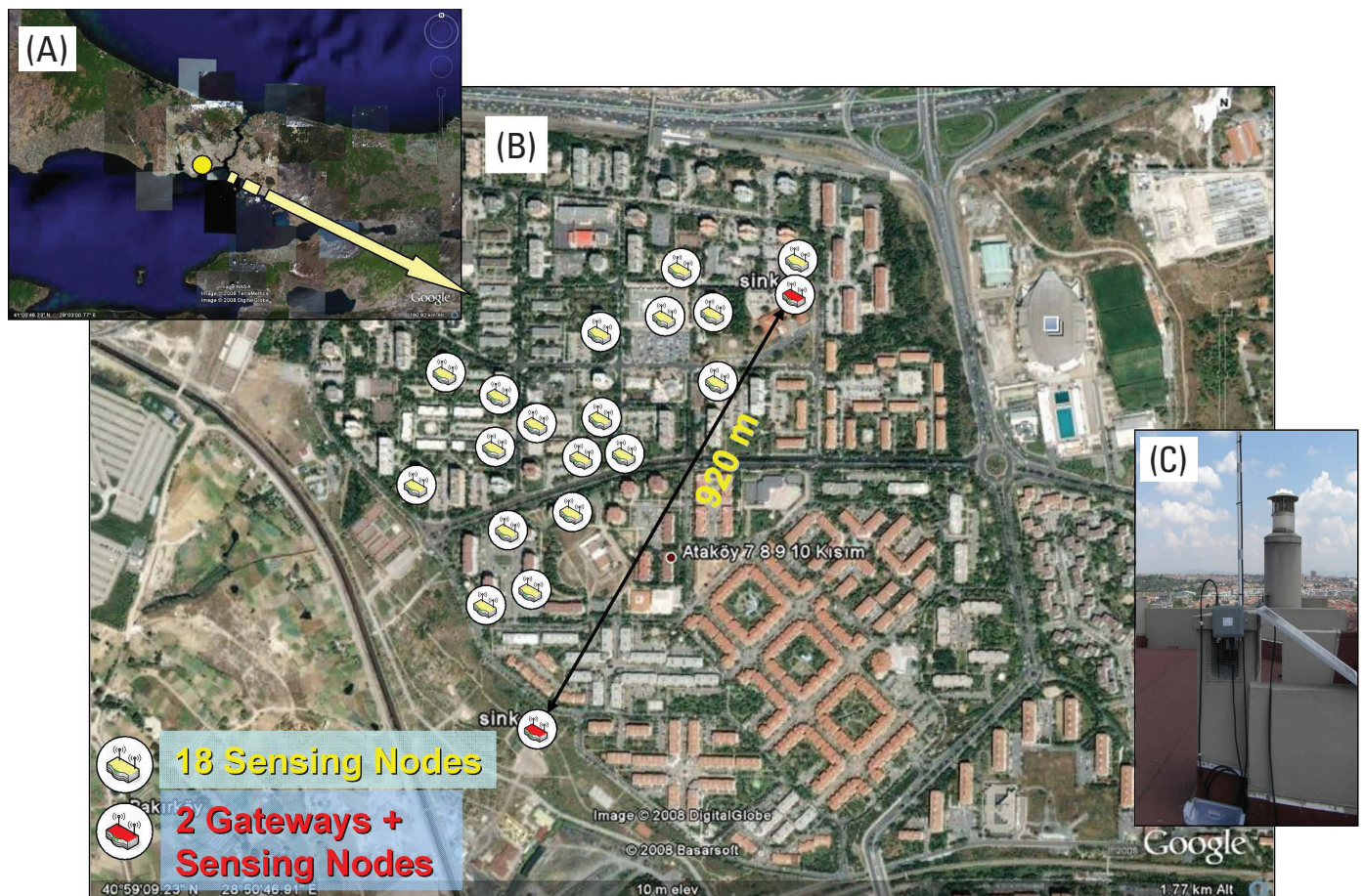
▲ Figure 7. (A) Location map of Istanbul showing the Ataköy district, where the test-bed SOSEWIN is situated. (B) The location of the sensing nodes and gateways for the test SOSEWIN in the Ataköy district, Istanbul. (C) A typical SOSEWIN sensing node installation.
