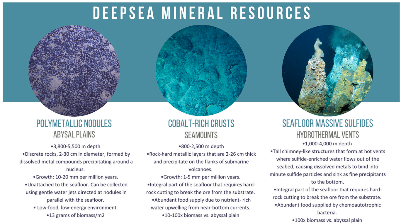
Fig. 2. Marine minerals studied in this article (edited from the TMC Impact Report, 2021). Credits: Polymetallic Nodules, TMC; Co-rich ferromanganese Crusts, Hino et al. (2023) , and Seafloor Massive Sulfides, Ishikawa et al. (2016) .
