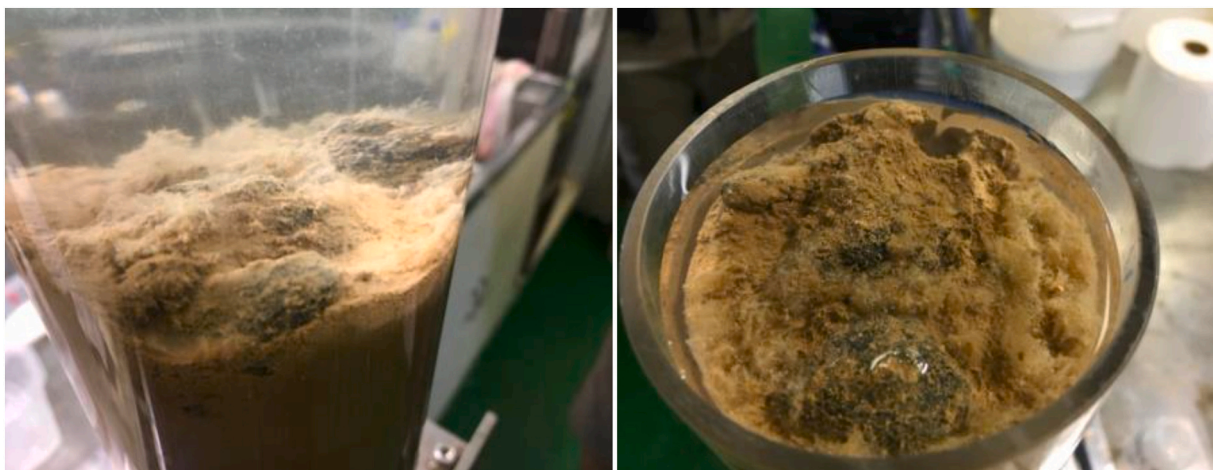
Fig. 5. New core samples of polymetallic nodules (PN) offshore San Ambrosio (~26°S). Left side: vertical view of the core-7. Right side: top sight of the core-4 showing the samples (Credits: Kinoshita, 2019).
