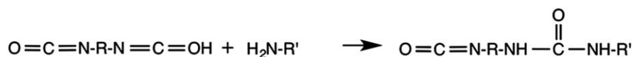
FIGURE 8. Tissue adhesion mechanism of urethane-based adhesive: \text{H}_2\text{N}-\text{R}' represent tissue amines that react with isocyanate groups through urea bond formation.
