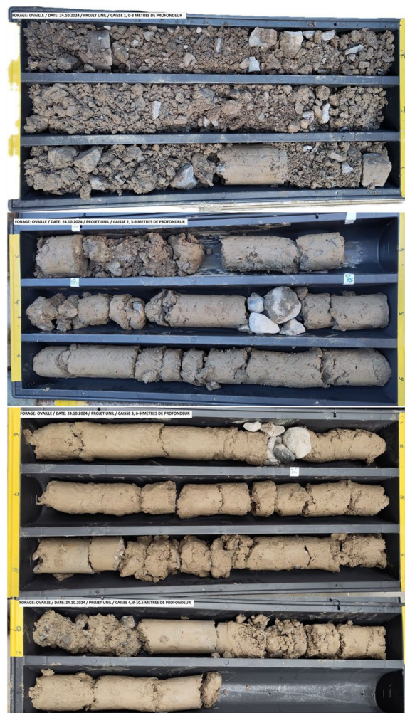
Fig. 2 Photos of drilled cores taken on site directly after drilling, in their fresh state. Each core box slot is 1 m long, and core sections follow one another left to right then top to bottom
