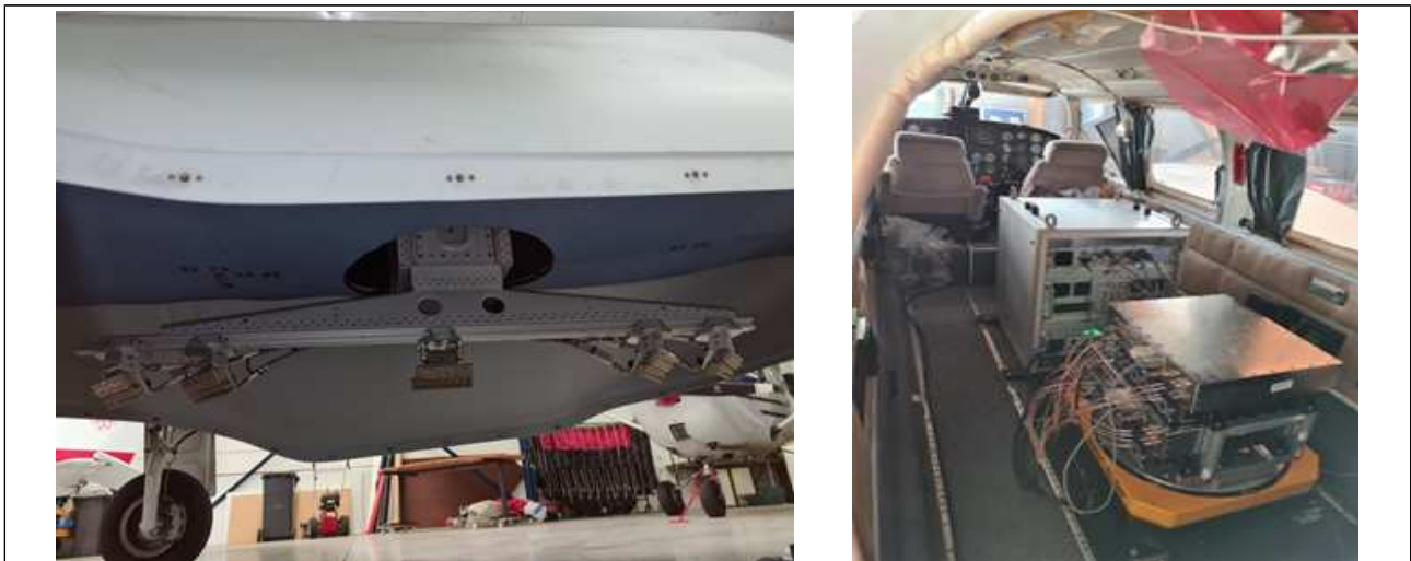
Figure 51. Antennas and instrument fixed on the aircraft.
