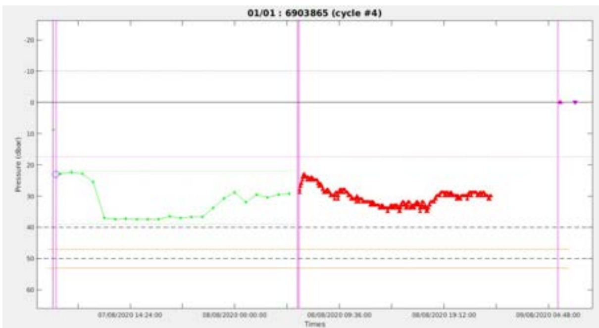
Figure 57. Underwater trajectory (time versus pressure figure) of the float WMO 6903865 for cycle 4. Coriolis DAC (Argo decoder nc_cycle_trace_times) Pump actions are depicted in red, suggesting the float had difficulties to ascend since its pressure did not decrease much.
