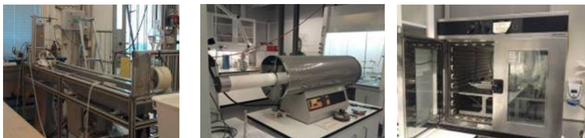
Pictures of the (1) spinning machine for hollow fiber fabrication and coating; (2), carbonization rig and (3) the pilot scale flat sheet coating device Photos ©NTNU, all rights reserved
