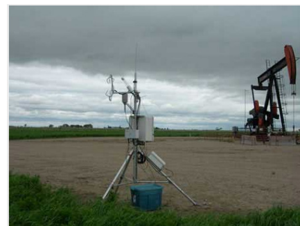
Continuous CO 2 and CO 2 flux measurement by eddy covariance. Click anywhere to close
