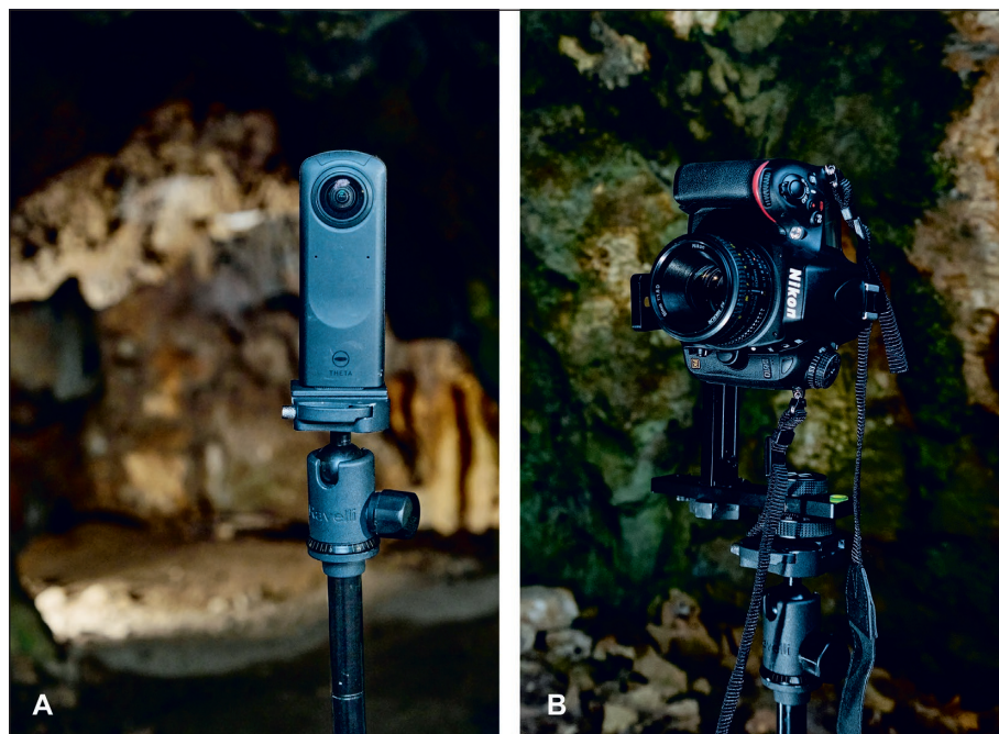
Figure 2: Photographic equipment used for the acquisition of the VT imagery: (a) Ricoh Theta Z1 360° camera, (b) Nikon D610 DSLR camera.
