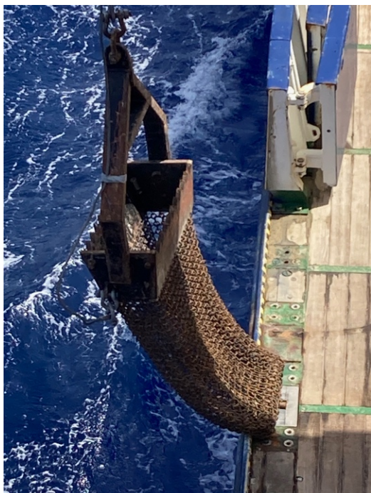
Fig. 5.18: Deployment of a chain bag dredge near the Italian island of Linosa.
