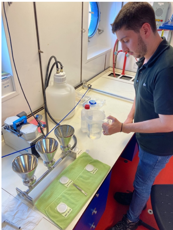
Fig. 5.23: Micropaleontologist O. Archontikes funnelling seawater through the filtration ramp.
