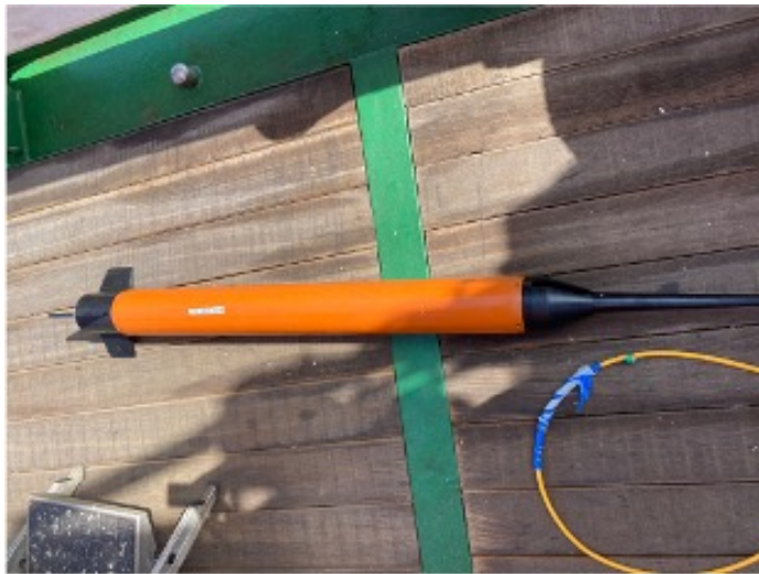
Fig. 5.12 (above): Towfish containing Overhauser magnetometer.
