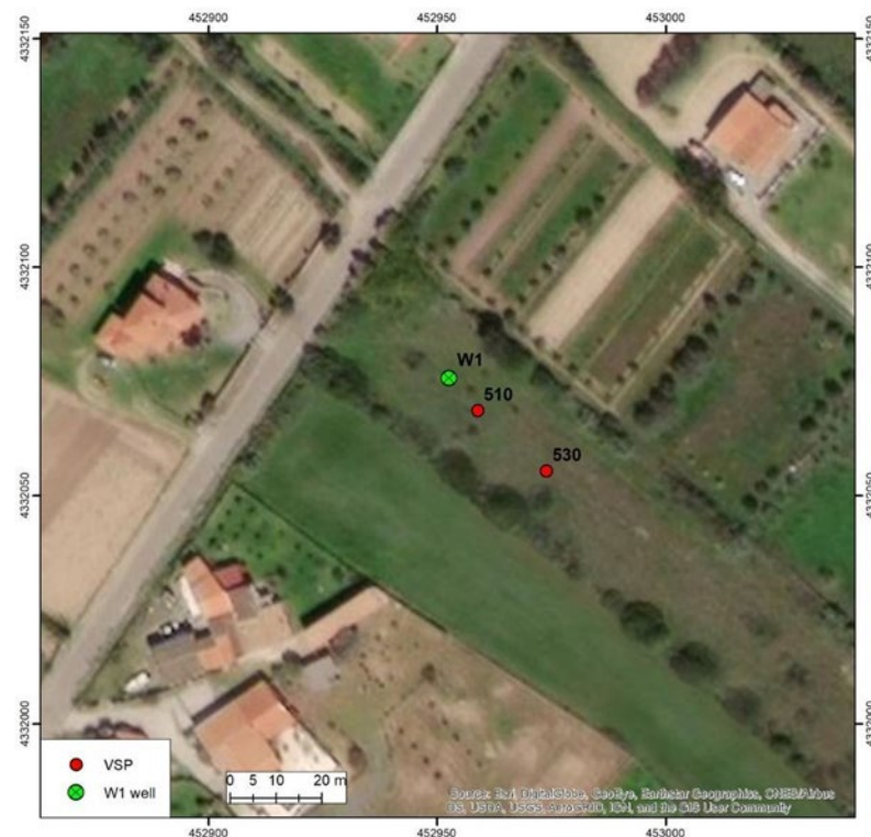
Figure 7. Map showing the position of the well W1 and the positions of the seismic source for the first near-offset VSP (Shot Point 510) and the second near-offset VSP (Shot Point 530).
