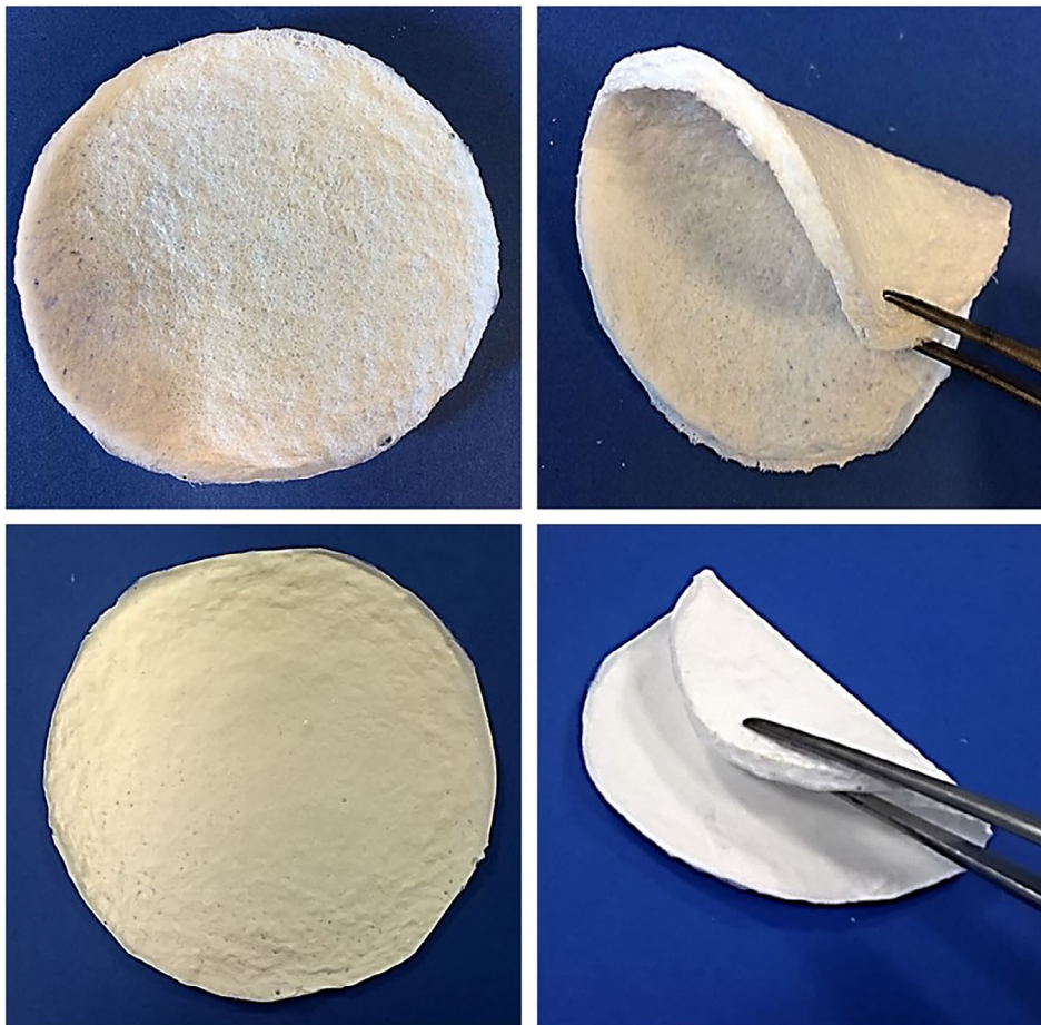
FIGURE 1 C2M membranes (upper row) and C3M membranes (lower row) reticulated with boric acid. The CTL-membrane displays a homogeneous texture and pliability. CTL, lactose-modified chitosan
