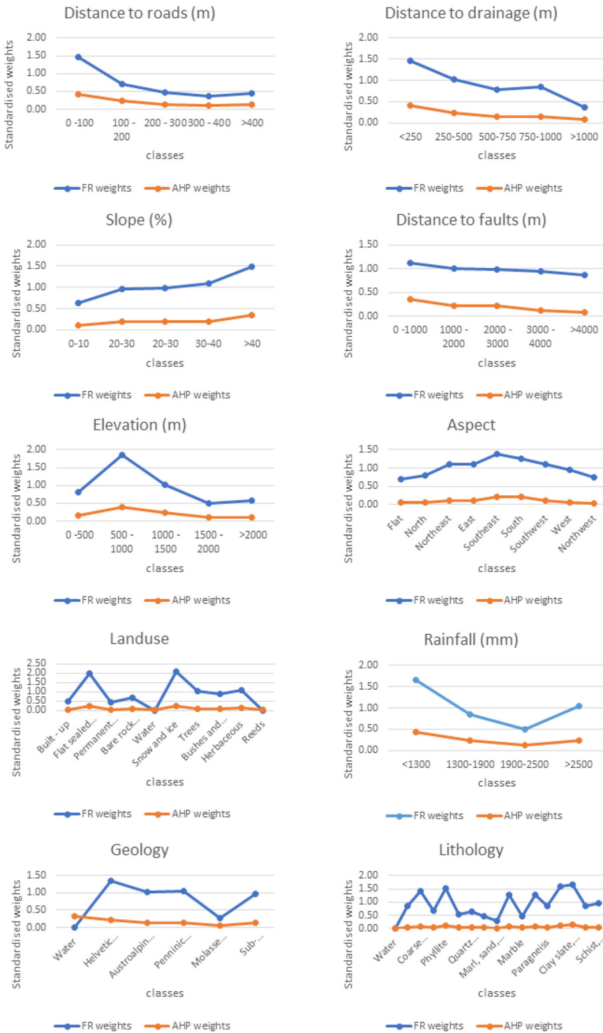
Figure 15. Comparison of the resulting weights for each factor and the classes based on the FR and AHP model.
