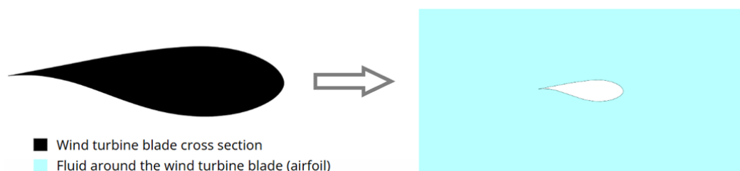
Figure 4.14. Fluid domain geometry.
