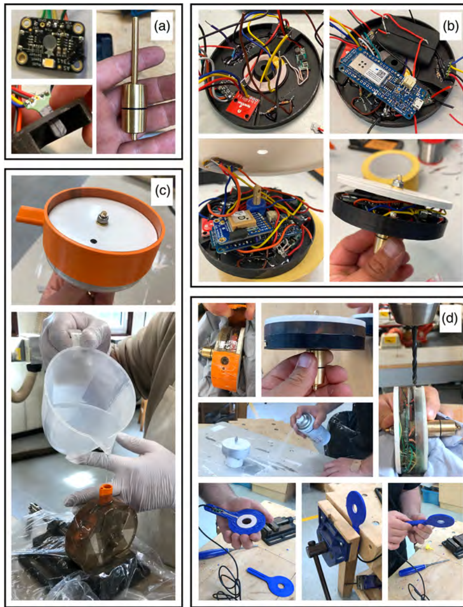
Fig. 2. Manufacturing the SSD. (a) Attaching diffuse glass to the spectral irradiance sensor (AS7341), coating the temperature sensor (TMP117) with thermally conductive epoxy and sinking it into the base of the device, and connecting the brass rod to the weight. (b) Building the device from bottom upwards, adding components and wiring. (c) Potting the device using the potting shell, sealing with tape and glue, and adding epoxy resin. (d) Removing the potting shell, drilling the magnet hole, spraying the disk, and manufacturing the wireless charger.
