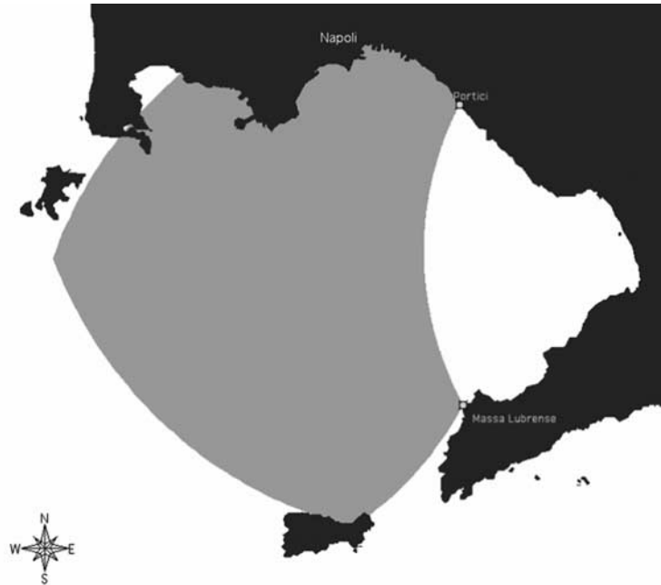
Fig. 2. – Coverage of the HF radar system in the Gulf of Naples, with the location of the two antennas (Portici and Massa Lubrense) and of the central site (Napoli).
