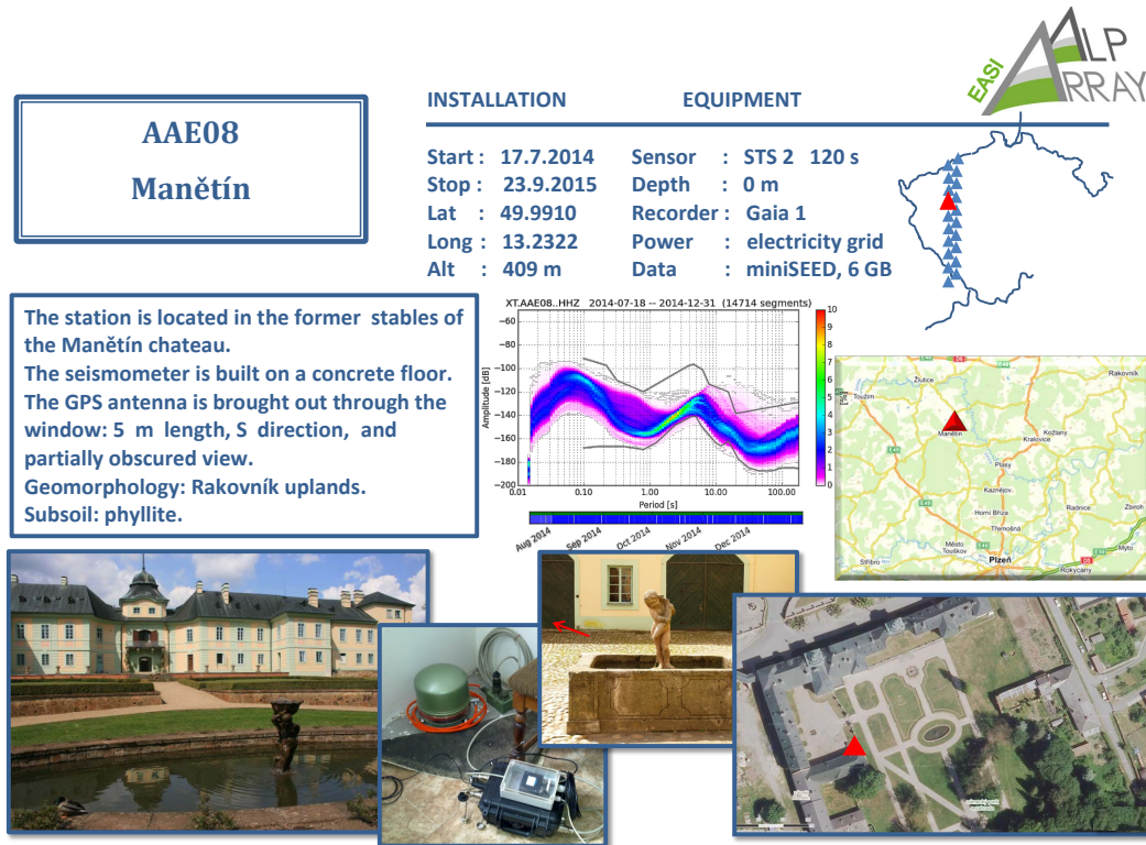
Figure 3. Example of installation of one of the broadband MOBNET stations in the AlpArray-EASI complementary experiment. In addition to the photo-documentation of the installation of the AAE08 station (Manětín), we show its location (upper right), station coordinates and period of recordings (top panel), and we describe the installation of accessories (GPS antenna) and the bedrock (left panel in the middle). The central panel shows the probabilistic power spectral density of ambient noise in the vertical component during the first 5 months of the station registration.
