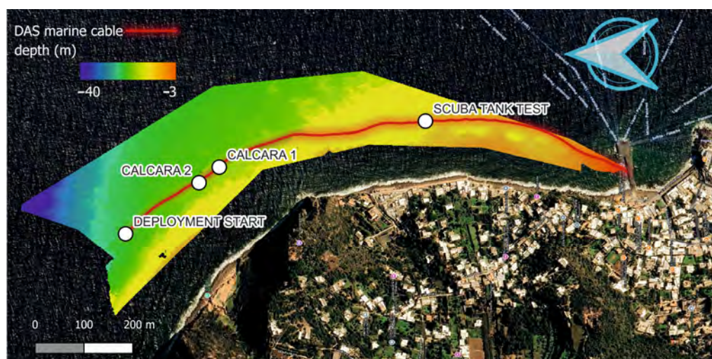
Figure 2. Deployment of the DAS cable laid down by the vessel offshore Panarea (red line). Relevant sites along the cable trajectory are indicated in the map, which includes bathymetric data of the surrounding area.
