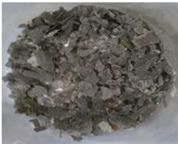
Figure 1: LCD scraps crushed with dimensions of about 10 mm
