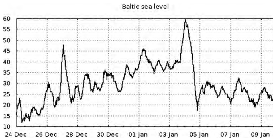
Figure 4.6.4. Observed sea level in the central Baltic Sea, calculated as an average of sea level at two central Baltic stations (Landsort Norra and Degerby) as derived from product ref. 4.6.3.
