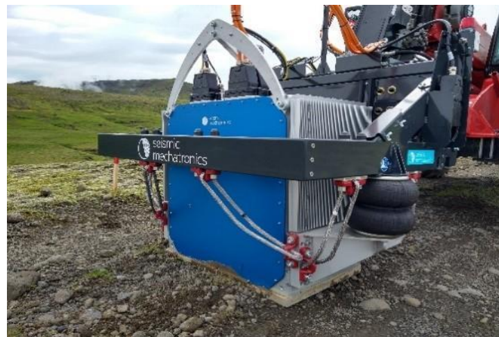
Figure 10. Electric seismic source (E-Vibe). Baseplate and reaction mass.
