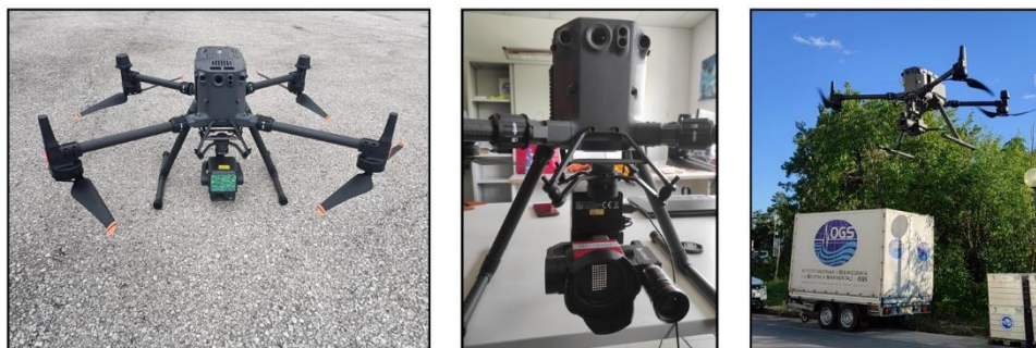
Figure 1 - Drone DJI Matrice 300, with (from left to right): laser DJI L2, Hyperspectral camera Cubert Ultris x20 plus and Foto/Video DJI P1.
