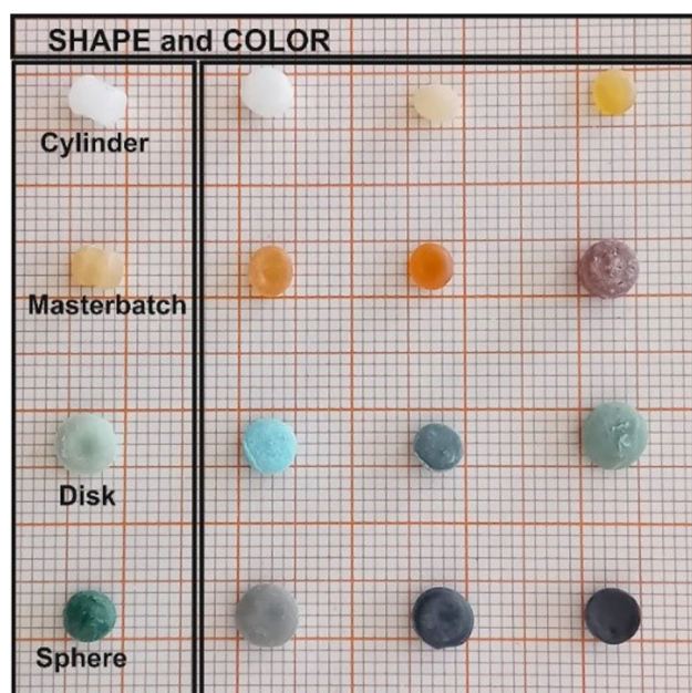
Fig. 2 Photos of plastic pellets collected on the beaches of the Aeolian archipelago. The selected particles show the different sizes, colors, and shapes representative of all the plastic pellets collected (Giugliano et al. 2022). White and light-yellow pellets accounted for most of the specimens found
