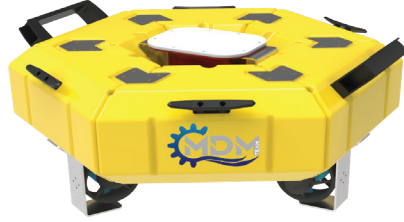
Fig. 1: The smart drifter prototype under construction. The modular structure allows fast assembly of parts in different possible conformations. The diameter is about 40cm.
