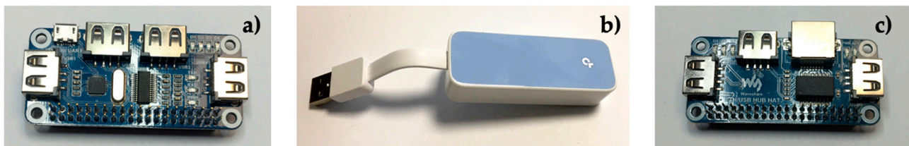
Figure S3. (a) Waveshare USB HUB hat with 4x extended USB 2.0 ports, (b) USB-ethernet adapter tp-link model UE200, (c) Waveshare ETH /USB hub hat.
