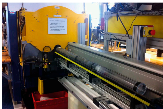
Figure F17. Natural Gamma Radiation Logger (NGRL).
