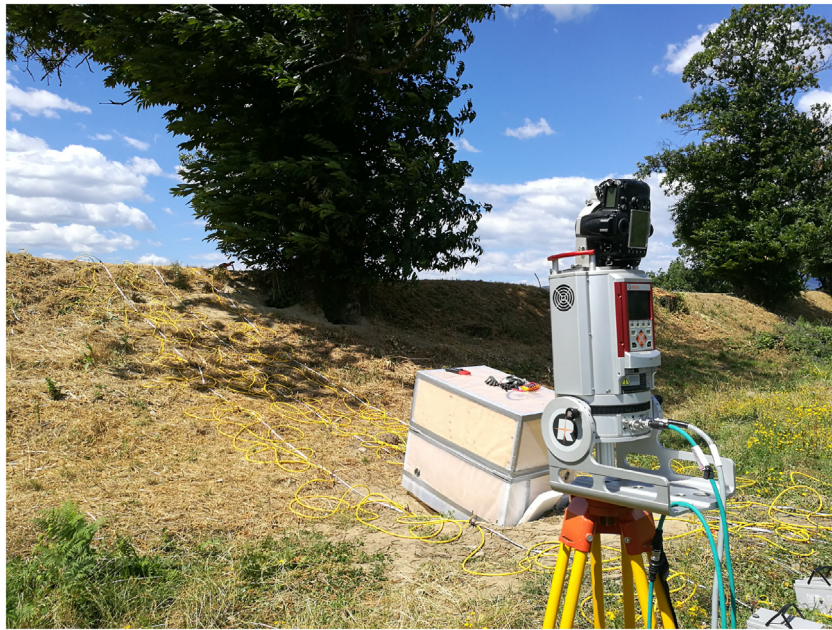
Fig. 2. Installation of MIMA (within the wooden box) in front of the levee body at the Bure creek. In this photo are also visible the TLS, on the front, and the ERT yellow cables, on the back.
