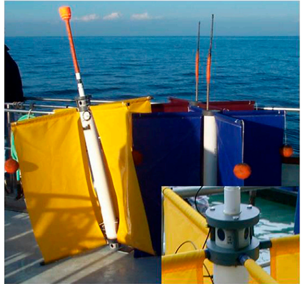
FIG. 1. (left) Prototype and (right) standard CODE drifters. The two Aquadopp velocimeters mounted at the top and bottom of the prototype drifter are clearly seen. The inset is an enlarged photograph of an Aquadopp velocimeter with transducers.
