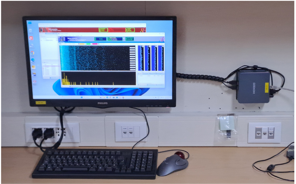
Fig. 3. PC station to operate the gamma-ray spectrometer and store the data.
