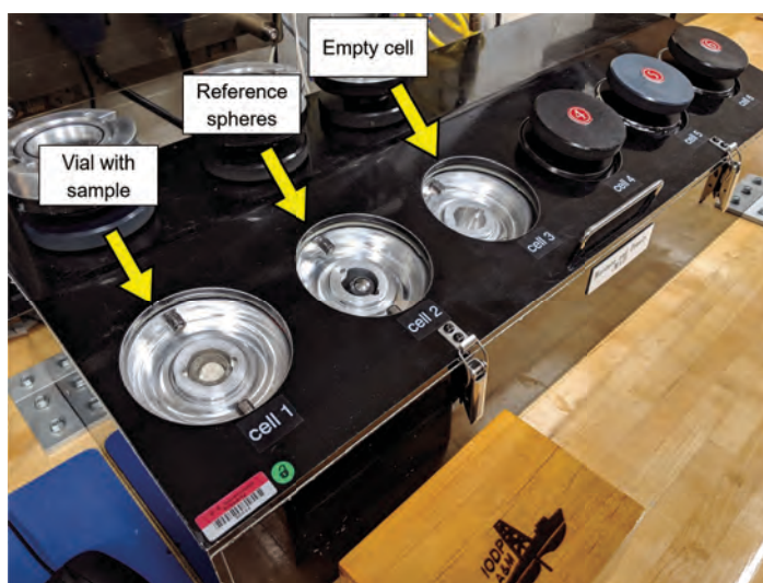
Figure F21. Pycnometer used to measure volume of dry samples for MAD analyses, Expedition 403.
