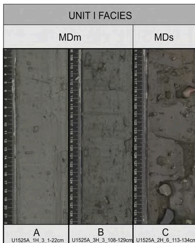
Fig. 5. Core images displaying facies in Unit I from: A) 3.01–3.22 mbsf; B) 22.19–22.4 mbsf and; C) 17.26–17.47 mbsf. Massive Muddy Diamict, MDm (A, B), displays varying amounts of clast content as demonstrated in A and B. C displays facies MDs.
