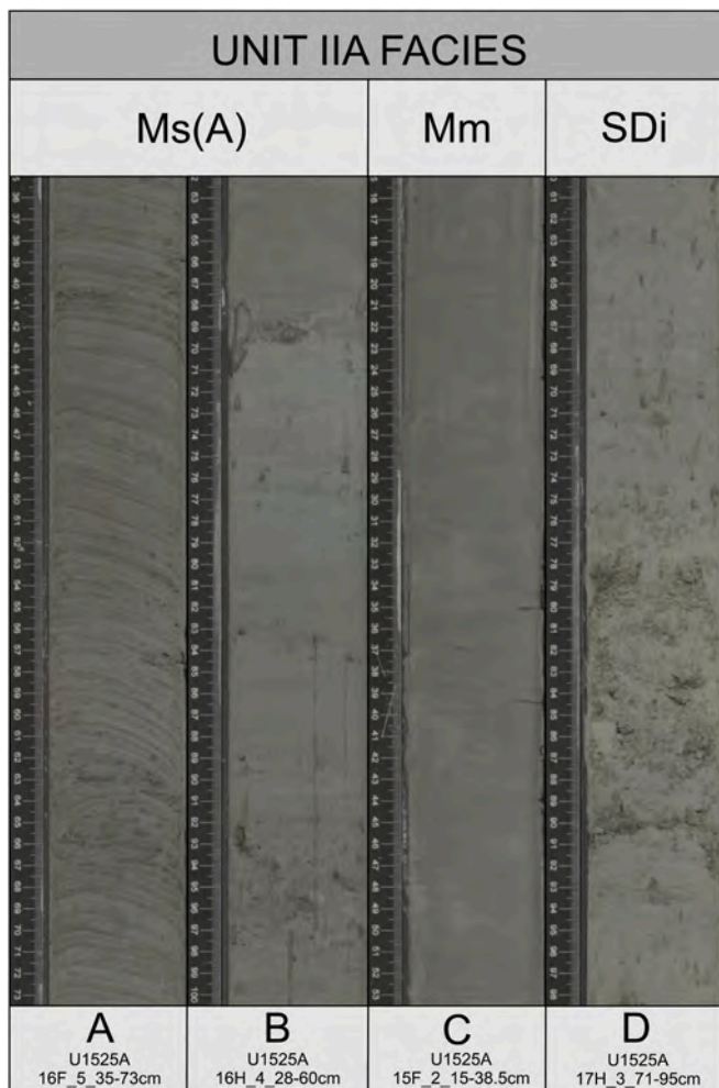
Fig. 6. Core images displaying facies in Subunit IIA from: A) 83.81–84.19 mbsf; B) 85.5–85.88 mbsf; C) 76.11–76.49 mbsf; D) 92.12–92.5 mbsf. Mode 1 and 2 of facies Ms(A) are shown in A) strongly Type A-interlaminated mud with silt laminae, and B) weakly Type A-laminated mud interbedded with cm-scale sandy muds or diamicts (see Table 1 for in-depth facies description). Images C and D show facies Mm and SDi, respectively.
