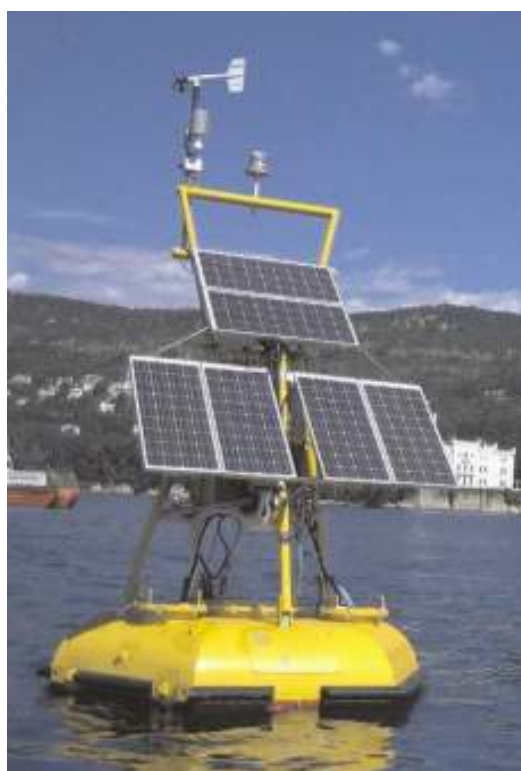
Fig. 2 - The new monitoring buoy in the offshore test position.
