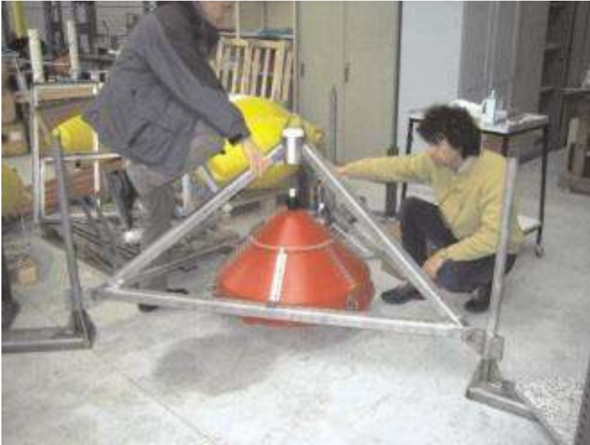
Fig. 3 - The gas sampling funnel in a tripod frame
