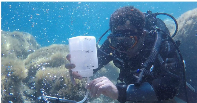
Fig 3. Measures of gas output flux from sediments by a INGV researcher at the San Giorgio vents.
