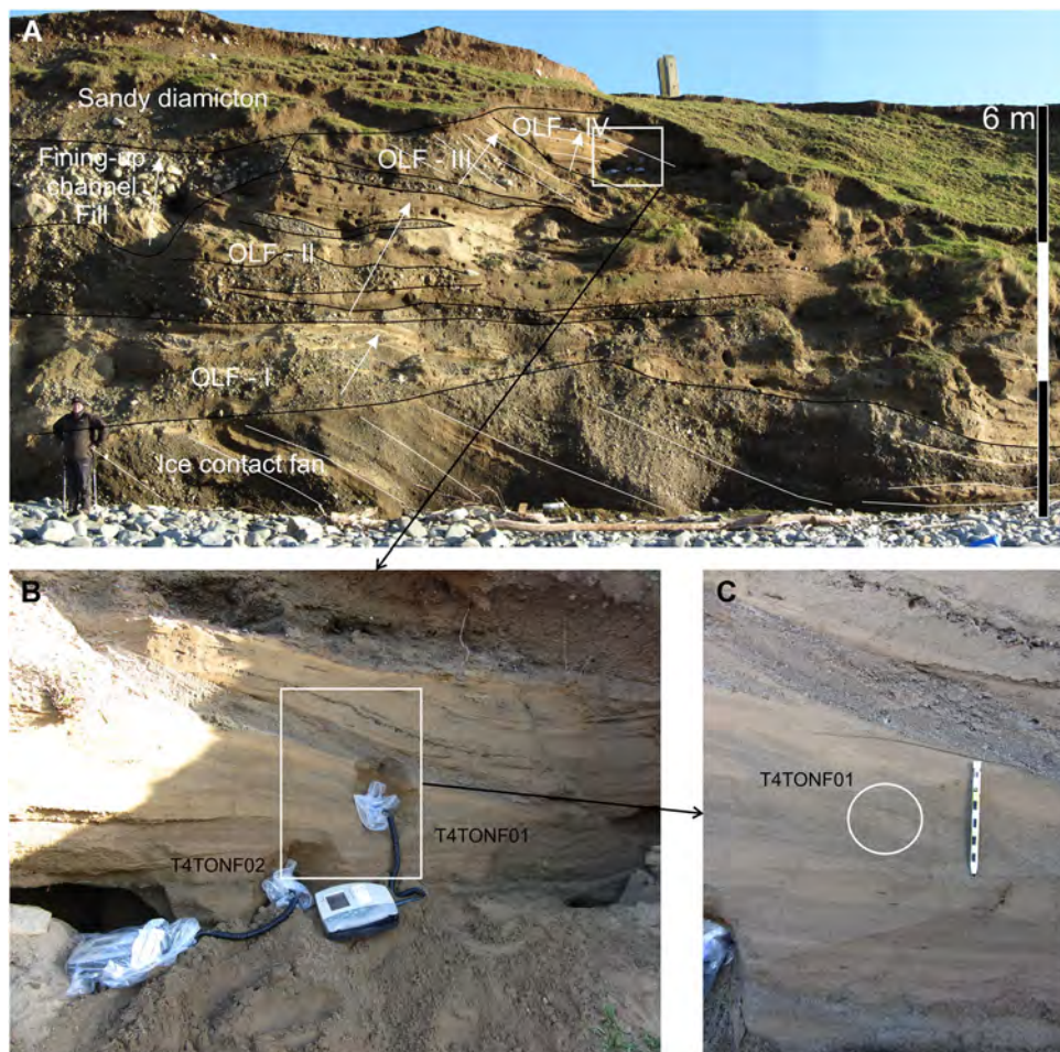
Figure 4. (A) Coastal section at Tonfanau sampled in December 2013 located 10 m north of the Log profile TON8 described by Patton and Hambrey (2009). The sequence comprises a steeply dipping basal package of ice-contact fan gravels with minor sand beds, buried by more horizontally bedded outwash lithofacies (OLF) OLF-I and OLF-II. Progressing up sequence, sand beds are increasingly dominant and OLF-III and IV dip more steeply to the south to south-west. (B) OLF-IV south-dipping beds of rippled coarse- to fine sand and the two samples collected. (C) Close-up of the sample T4TONF01 measured for OSL. For full description and interpretation of the Tonfanau sections see Patton and Hambrey (2009). [Color figure can be viewed at wileyonlinelibrary.com ].
