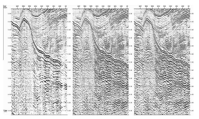
Fig. 3. Original scanned seismic section converted to SEG-Y (left). Same data processed to correct amplitude anomalies from the scanning process and restore continuity of the signal using the Tau-P transform (center). Final migrated section (right).
