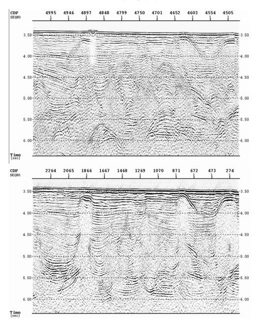
Fig. 6. Comparison of migrated seismic section showing diapiric structures without reprocessing (upper section) and with reprocessing (lower section).
