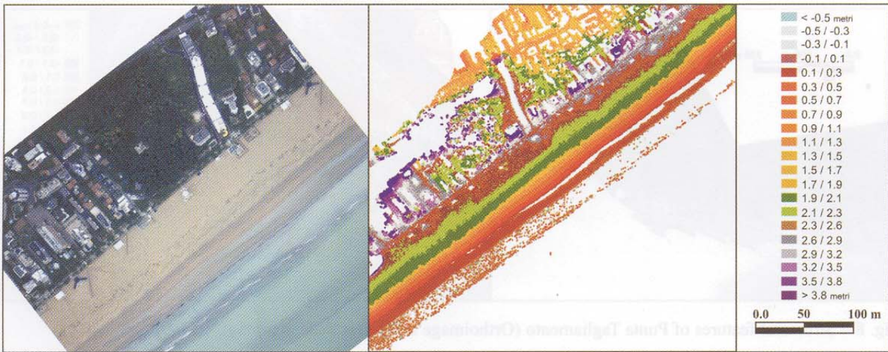
Fig. 6 - Orthoimage and Laser Scan mapping acquired in correspondence to the Lignano Sabbiadoro shore; the backshore and foreshore in this coastal sector highlight the maximum extension.
