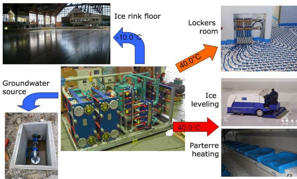
Figure 16. Working scheme for heating and cooling of Pontebba open loop heat pump plant.
