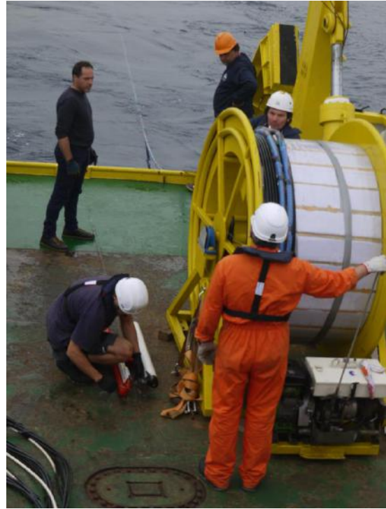
Figure 17. The hydrophone streamer release operations during the MCS survey on board the R/V “Aegaeo”.
