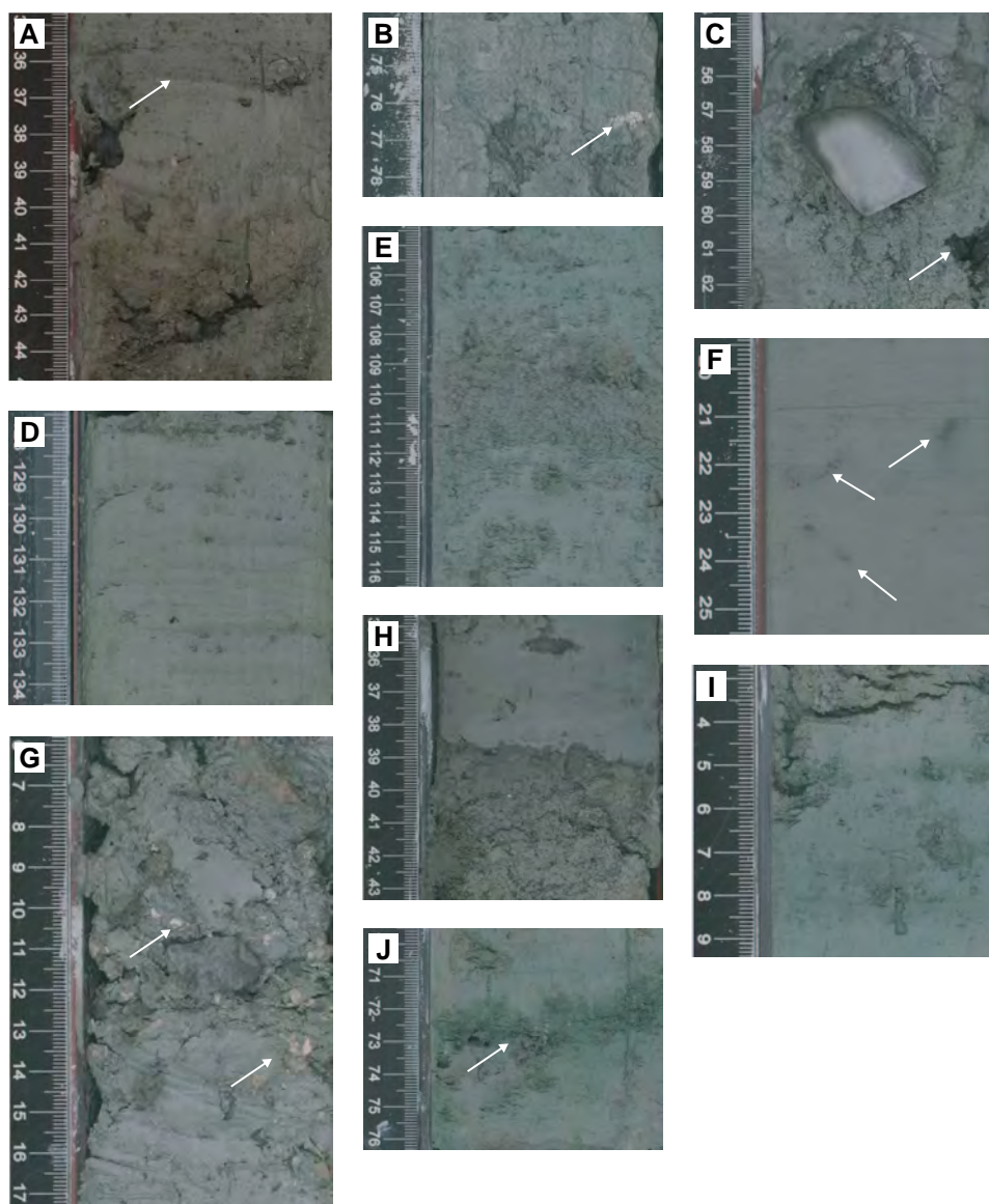
Figure F7. Sedimentary structures and diagenetic features, Site U1523. A. Sharp contact (white arrow) between diatom-bearing mud and sand (Unit I; U1523E-3F-2A, 37 cm). B. Shell fragments (white arrow) (Unit I; U1523A-2H-2A, 76–77 cm). C. Lignite clast with organic material (white arrow) in a diamict (Unit I; U1523E-4F-2A, 55–63 cm). D. Laminations in diatom-rich mud (Unit II; U1523B-7F-3A, 128–134 cm). E. Bioturbated contact between diatom-bearing sand and mud (Unit II; U1523E-12F-2A, 105–116 cm). F. Pyrite-filled burrows (white arrows) in mud (Unit III; U1523B-20F-2A, 20–25 cm). G. Shells (white arrows) in diamict (Unit II; U1523E-15F-2A, 6–17 cm). H. Sharp contact between sand and mud (Unit III; U1523E-20F-1A, 38–39 cm). I. Glauconite staining (Unit III; U1523E-20F-3A, 3–9 cm). J. Glauconite staining (Unit III; U1523E-20F-3A, 70–76 cm; white arrow).
