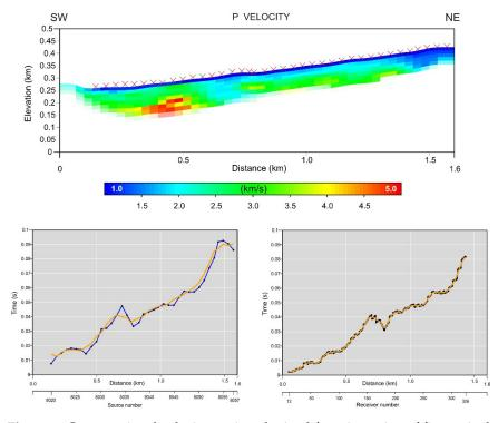
**Figure 9.** Compressional velocity section obtained from inversion of first arrivals (top), using the simultaneous iterative reconstruction technique (SIRT) algorithm [52]. Red crosses are the shot points. The bottom panels show the smoothed applied static corrections (yellow solid line) and punctual static corrections (blue) for sources (left) and receivers (right), respectively.
