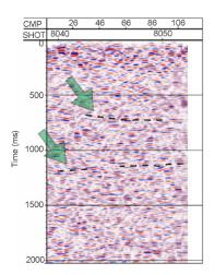
**Figure 16.** Band-pass-filtered (5-16-45-50 Hz) stacked time section, with post-stack mix of the TUD data (vertical component) and AGC for visualisation purposes. The green arrows and the dashed lines indicate the expected reservoirs in two-way travel time.
