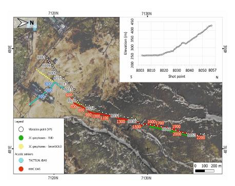
**Figure 2.** Surface seismic monitoring layout. Line/geometry overview (2C TUD geophones are 20 m down-shifted for display purposes only). The topographic profile of the shot point line is shown in the top-right corner. The map coordinate system is WGS 84/UTM zone 27 N in km.
