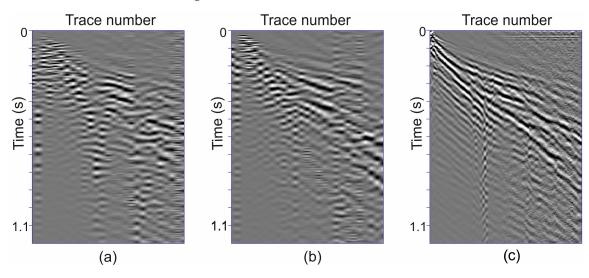
**Figure 4.** (**a**) In-line horizontal component of SmartSolo<sup>®</sup> geophones, (**b**) their vertical component and (**c**) the HWC DAS signal for the vibration point 8041.
