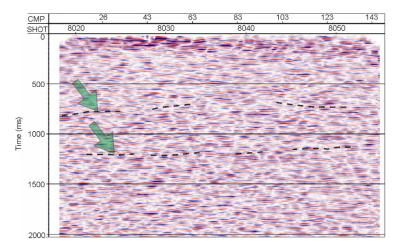
**Figure 15.** Band-pass-filtered (5-16-45-50 Hz) stacked time section, with post-stack mix and AGC for visualisation purposes, of the SmartSolo<sup>®</sup> data (vertical component). The green arrows and the dashed lines indicate the expected reservoirs in two-way travel time.
