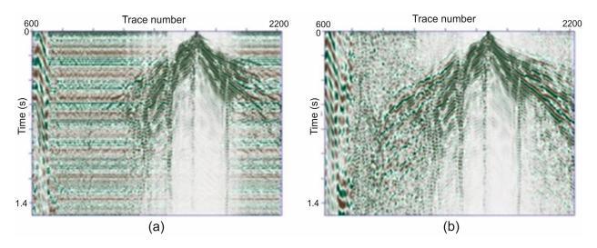
**Figure 8.** (a) Common-shot gather 8041 from HWC DAS recordings affected by optical noise (horizontal stripes). (b) The same shot gather after optical noise removal and signal recovery. Data are not filtered.
