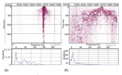
**Figure 12.** SmartSolo<sup>®</sup>s common-shot (**top**) for the common-shot gather 8041 before (**a**) and after (**b**) balancing. The blue lines in the bottom of the figures are the corresponding frequency spectra.
