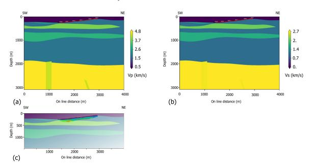
**Figure 6.** SW-NE-oriented models: (**a**) final compressional velocity model; (**b**) shear velocity model updated using the results from the laboratory transmission experiments. (**c**) A blow-up of the shallower part of the model (up to about 1500 m depth) in (**a**) with the superimposed result of the first-break tomography. The velocity scale is the same as in (**a**), but a transparency has been applied to highlight the superimposed result.
