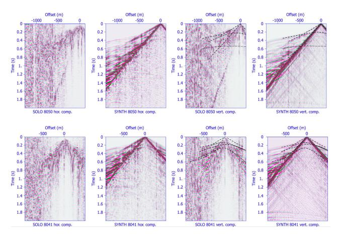
**Figure 7.** Common-shot gathers: comparison between the horizontal and vertical components of the SmartSolo<sup>®</sup> geophones and the corresponding synthetic particle velocity components for shots 8050 (**top**) and 8041 (**bottom**). Synthetic data are computed using the velocity models of Figure 6a and a vertical point source with a 20 Hz peak frequency. As an example, the dotted lines in the vertical components of the shots highlight the qualitative similar trends of selected events.
