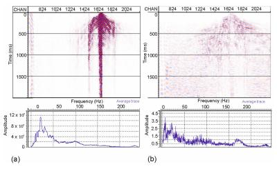
we applied a time exponential power of 1 to recover the spherical divergence in the seismic signals at higher times (Figure 10).
