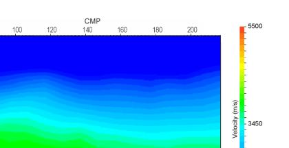
**Figure 11.** 2D stacking velocity section calculated from the HWC DAS dataset.
